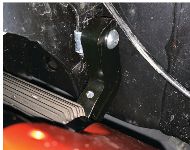
Fig. 26: Mount the bracket to the body mount.
