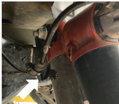
Fig. 42: Un-indexed coil wire.
