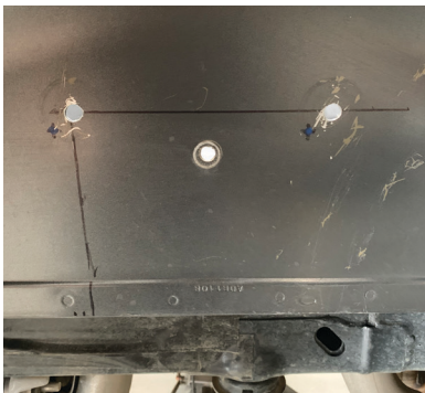
Fig. 50: Drill holes for cooler.
