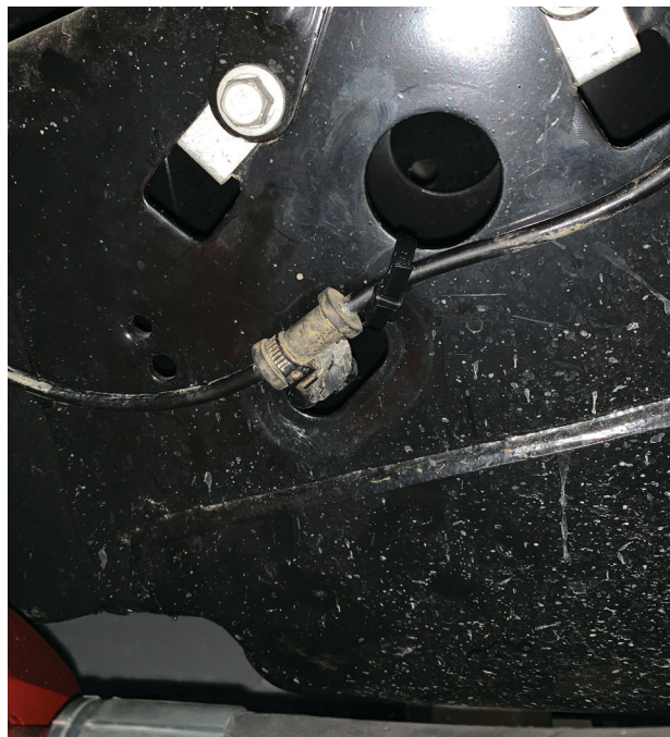
Fig. 32: Secure the coil wire.
