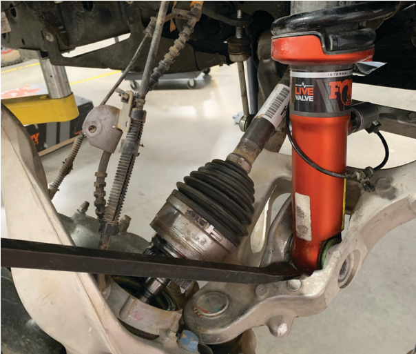
Fig. 16: Remove the shock.
