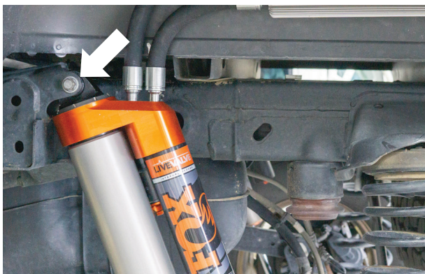
Fig. 53: Install the upper shock bolt (driver side shown).
