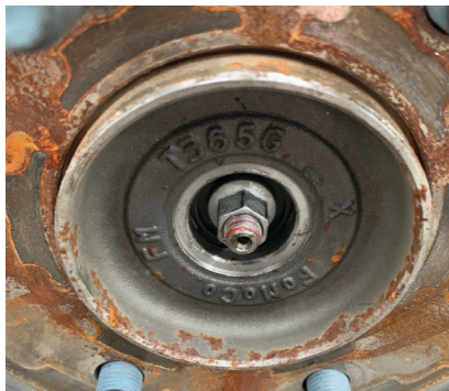
Fig. 37: Install the CV axle nut.
