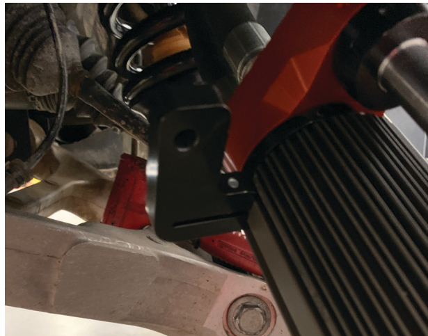
Fig. 25: Torque bolts to 18 ft-lbs.
