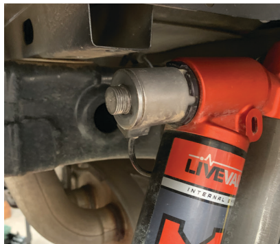
Fig. 44: Remove coil cap.
