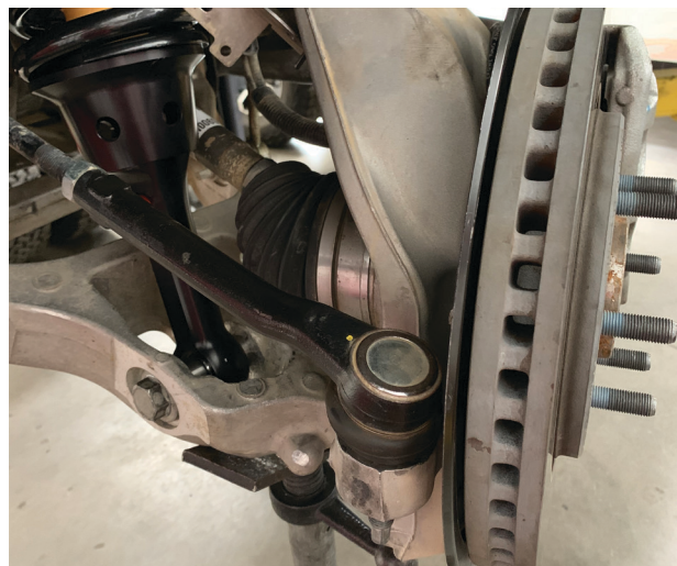
Fig. 35: Re-index the CV axle.
