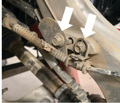
Fig. 4: Wires attached to the spindle.
