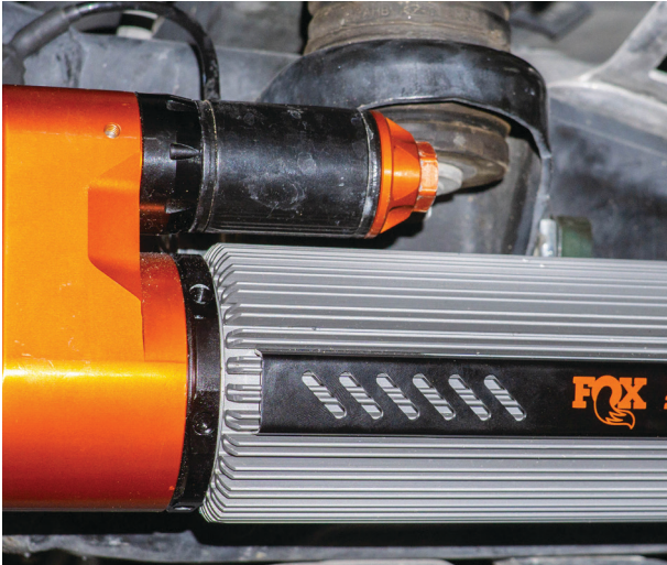
Fig. 29: Tighten the coil cap.
