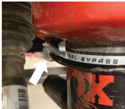
Fig. 12: Unindex coil wires.
