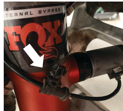
Fig. 13: Unindex coil wires.
