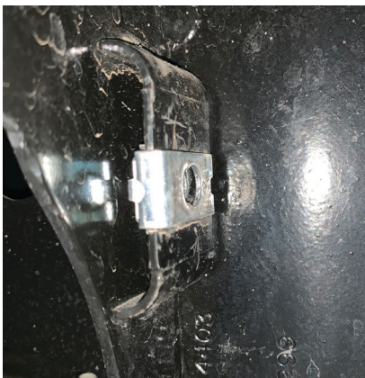
Fig. 23: Install clip nuts.
