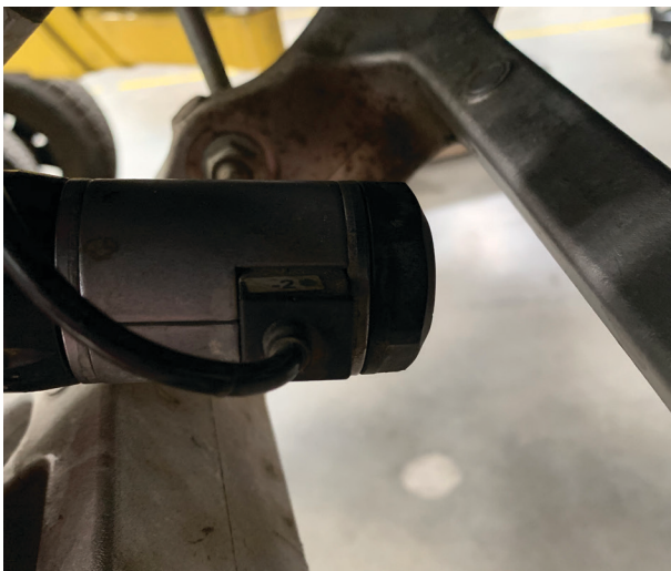
Fig. 14: Remove the Live Valve coil cap.
