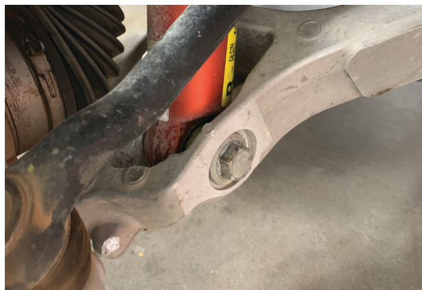
Fig. 2: Remove the lower control arm bolt.
