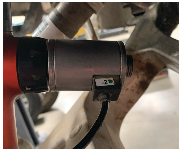
Fig. 15: Remove the Live Valve coil cap.
