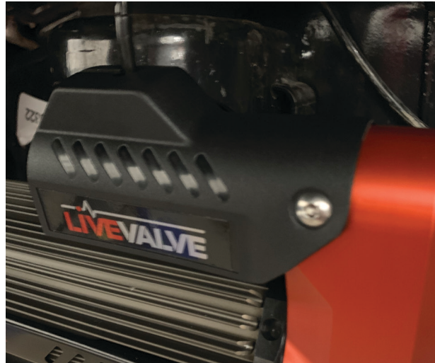
Fig. 30: The Live Valve decal faces outward.
