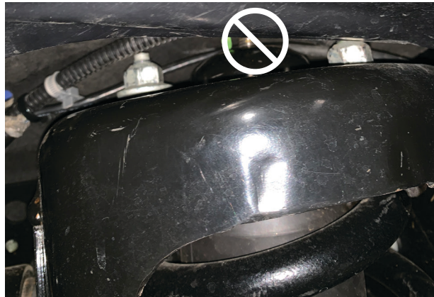
Fig. 1: Remove the three top hat nuts.
