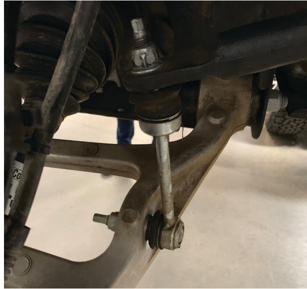
Fig. 39: Install the sway bar.
