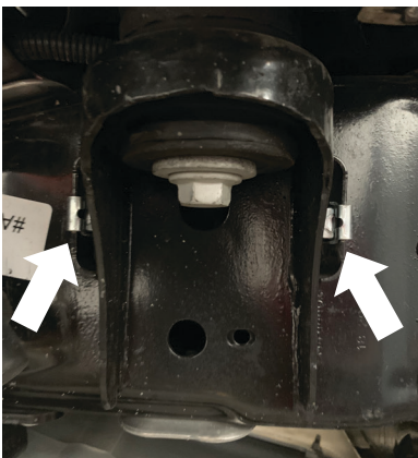
Fig. 22: Install clip nuts.
