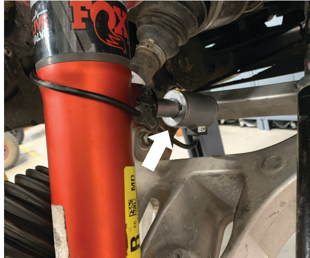
Fig. 17: Slide the Live Valve coil off.
