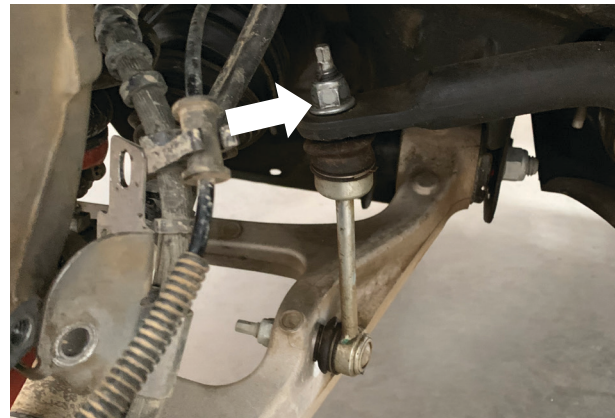
Fig. 6: Remove the sway bar from the end link.
