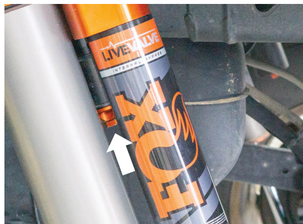
Fig. 58: Tighten the coil cap.
