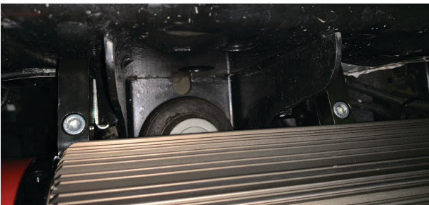
Fig. 27: Torque the pinch bolts to spec.
