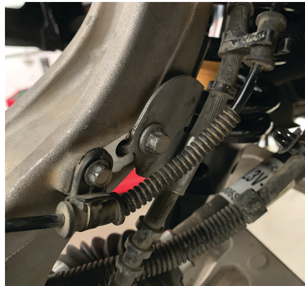
Fig. 40: Fasten wires to the knuckle.
