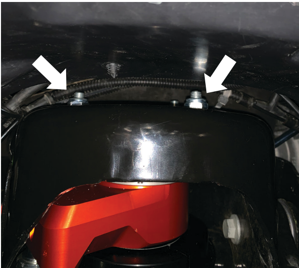
Fig. 20: Torque nuts to 24 ft-lbs.
