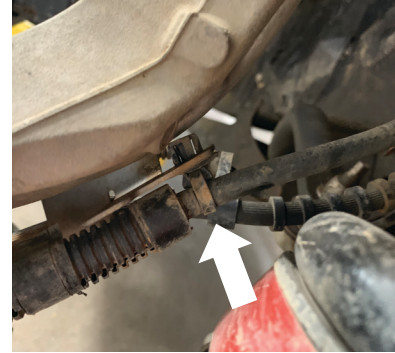
Fig. 5: Wires attached to the spindle.
