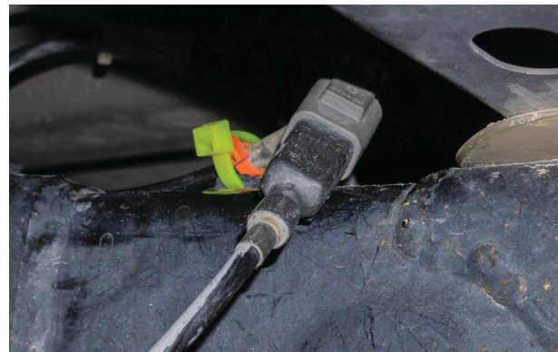
Fig. 60: Zip tie the Live Valve wire.
