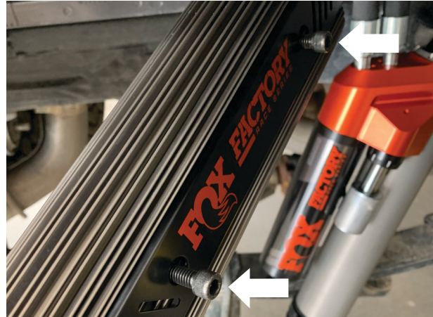
Fig. 56: Install the bolts.
