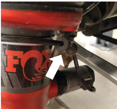
Fig. 11: Unindex coil wires.
